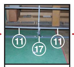
Line up pre-drilled holes and secure with bolt for parts 11, 10 and 17 following the image above. Repeat on the other side.
