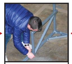
Line up pre-drilled holes and secure with bolt for parts 10, and 4 following the image above.
