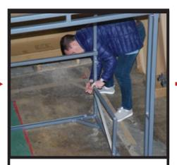
Line up pre-drilled holes and secure with bolt for parts 9, and 5 following the image above.
